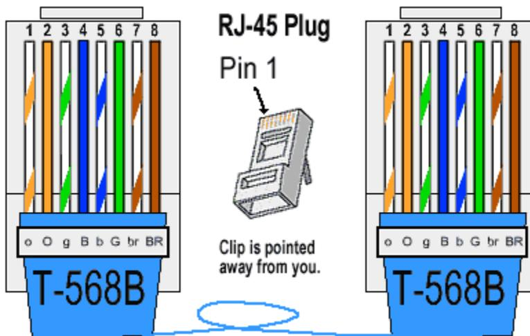
Both the T-568A and the T-568B standard Straight-Through cables are used most often as patch cords for your Ethernet connections. If you require a cable to connect two Ethernet devices directly together without a hub or when you connect two hubs together, you will need to use a Crossover cable instead.
